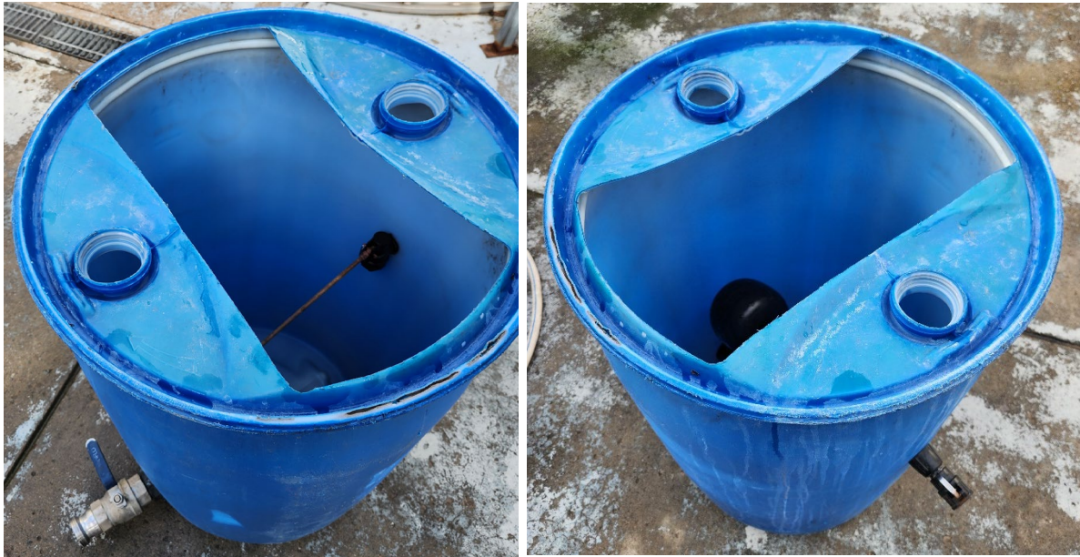
Figure 1 200L reused chemical drums reused for winery cleaning. A float switch has been installed at 100L level to reduce the amount of water used at each wash cycle.
